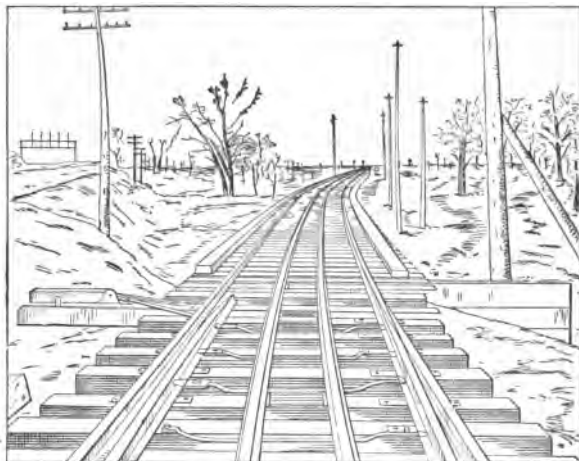
FIG. 106. Sectional Rail Installation.
