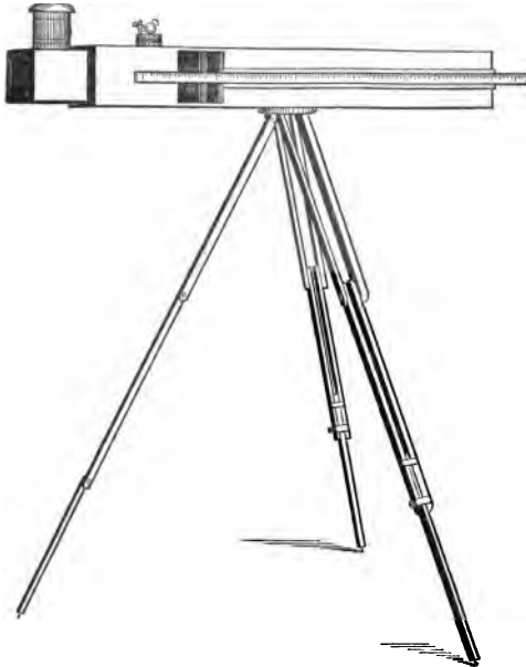
FIG. 1. Portable Bunsen Photometer.
