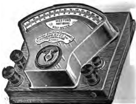
Weston Standard Portable, Direct Reading Voltmeter.
