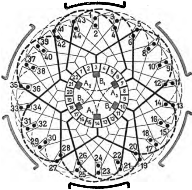
Six-pole drum simplex wave winding. Number of half-coils (which takes the place of Z in the theory of the winding) = 44, front pitch = + 7, back pitch = + 7, commutator pitch = + 7, throw of coils = 3, number of paths = 2.
