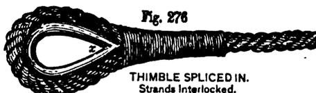
as shown at *a*. The other style (Fig. 276) is by interlocking the strands in the usual manner of splicing, and also wrapping with wire as in the first method; the latter mode of fastening possessing the greater strength.
