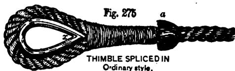
Two styles of splices are used: one (Fig. 275) in which the wires after being frayed out at the end, and the rope bent around the thimble, are laid snugly about the main portion of the rope and securely fastened by serving or wrapping with stout wire; the extreme ends which project below this wrapper being folded back,
