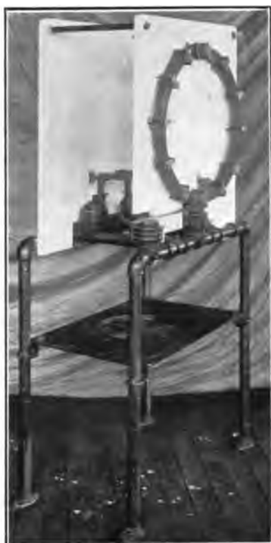
FIG. 9 High-speed air cooled fuse holder with magnetic blow-out used in test.
