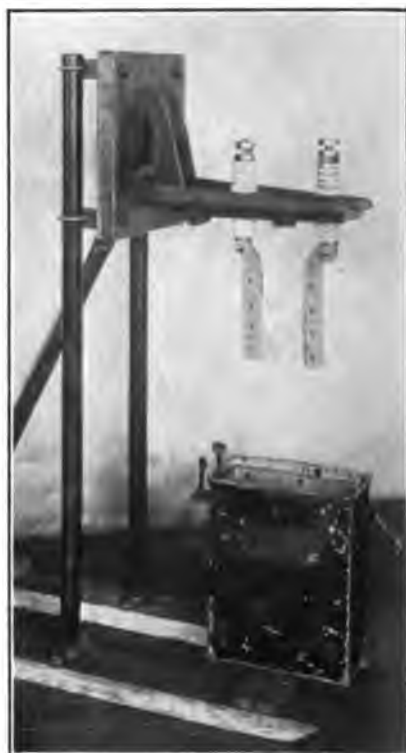
FIG. 10 High-speed oil-cooled fuse holder, used in test.
