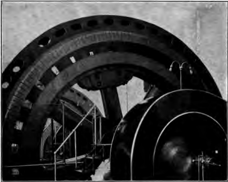
FIG. 194.—REVOLVING FIELD OF No. 2 ENGINE SHOWING COUNTERWEIGHT.
