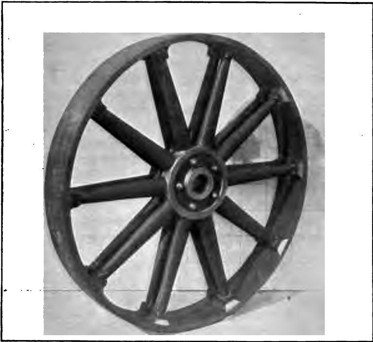
FIG. 74.—CAST-STEEL MODEL WHEEL.
