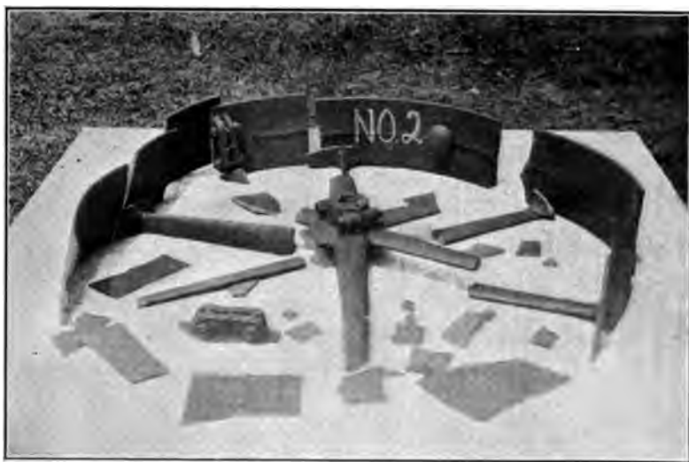
FIG. 70.—WHEEL NO. 2 AFTER BREAKING.
